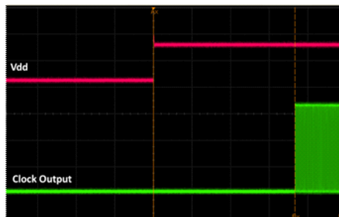
Figure 16. Startup Waveform vs. Vdd
